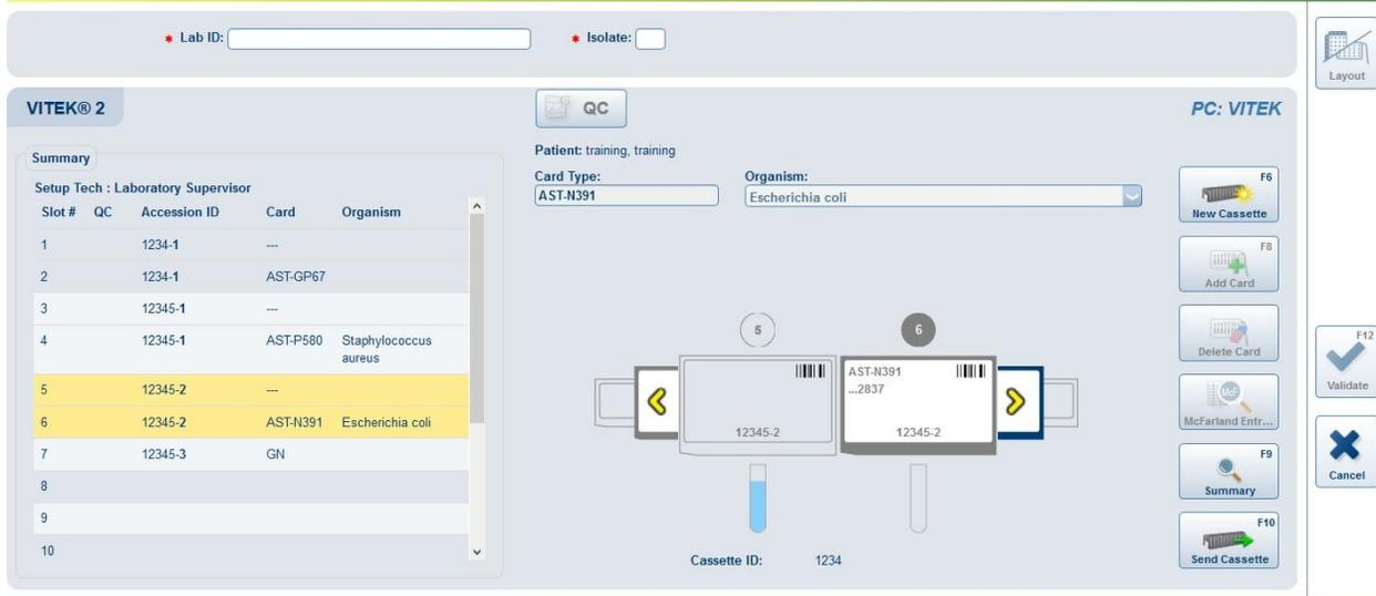
The screenshot shows the VITEK2 software interface. On the left is a 'Summary' table with columns for Slot #, QC, Accession ID, Card, and Organism. Slot 5 is highlighted. In the center, there is a diagram of a cassette with two slots, labeled 5 and 6, and a 'Cassette ID: 1234' below it. On the right, there are several function buttons: F6 New Cassette, F8 Add Card, F12 Validate, F9 Summary, and F10 Send Cassette. The top of the interface includes fields for 'Lab ID' and 'Isolate'.
