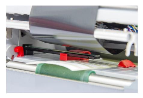
7. Move guides closely to the edges of the material without clamping the material.
