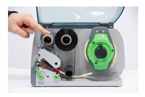
8. Turn transfer ribbon take-up hub counterclockwise to smooth out the feed path of the transfer ribbon.
