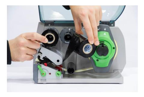
3. Get the set for transfer ribbon replacement, which is composed by a transfer roll and a ribbon core.
