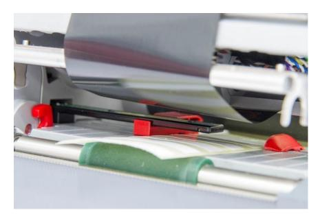
7. Secure starting end of the transfer ribbon to the ribbon core using adhesive tape.
