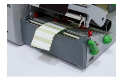
11. Press print head retainer down and turn lever clockwise to lock the printhead.
